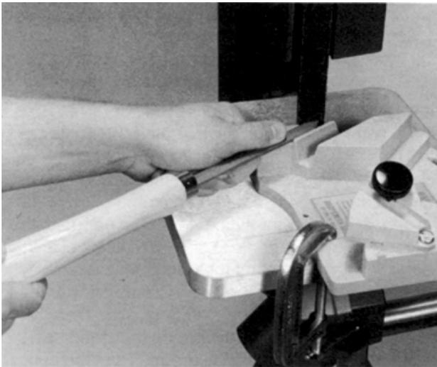
**Figure 24-13.** Set the parting tool's side in the first station.
