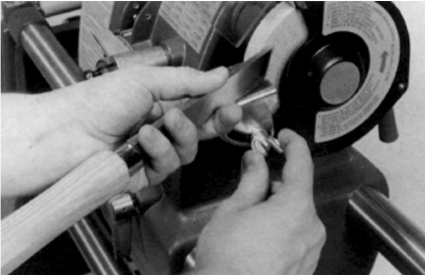
**Figure 24-15.** Hold the skew on the tool rest with the tip up and the bevel against the wheel.
