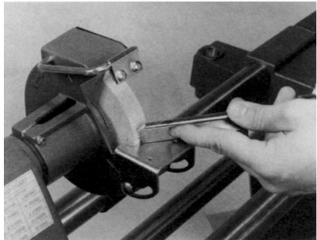
**Figure 24-19.** Roll the gouge to the front of the tool rest, this time with the handle pointing to the right.
