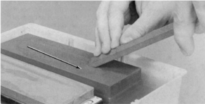
**Figure 24-29.** Point the cutting edge away from the direction you are sliding the tool.
