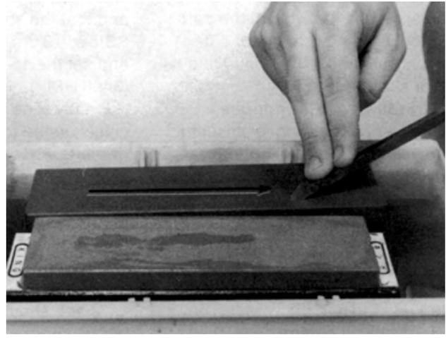
**Figure 24-24.** For narrow chisels, point the cutting edge away from the direction you are sliding the skew.
