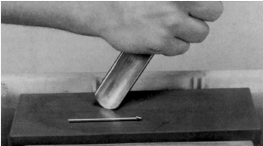
**Figure 24-27.** Point and roll the cutting edge away from the direction you are sliding the gouge.
