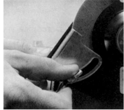
**Figure 24-32.** Set the angle so that the wheel is coned on the flat bevel. Tighten the wing nut securely.
