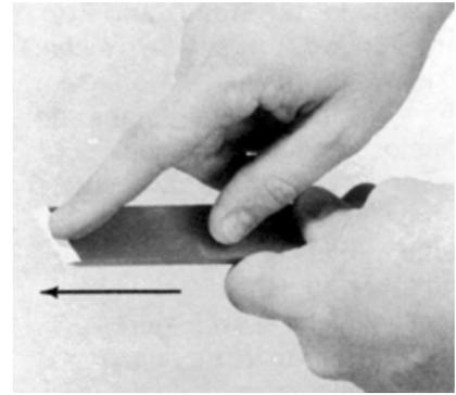
**Figure 24-22.** Feel the burr by carefully rubbing your finger toward the cutting edge.
