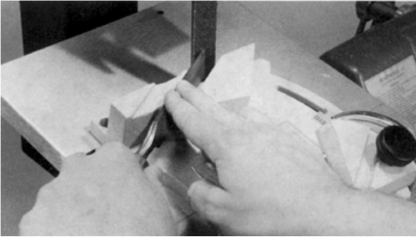
**Figure 24-31.** Slide the bench chisel into the abrasive. Hold the chisel there momentarily, then back it away.
