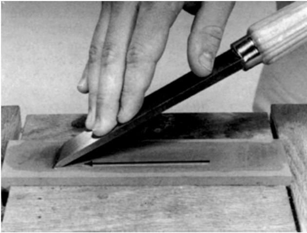
**Figure 24-23.** Point the cutting edge in the same direction you are sliding the skew.
