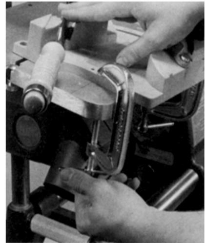
**Figure 24-30.** Position the sharpening guide within 1/16" of the belt and clamp it to the table.
