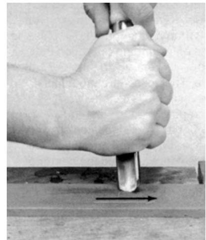
**Figure 24-25.** Point and roll the outside of the cutting edge in the same direction you are pushing the gouge.
