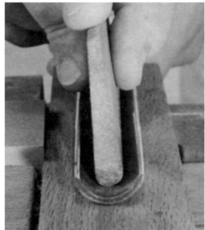
**Figure 24-26.** Use a rounded slip to hone the inside of the gouge.
