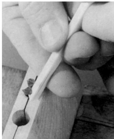
**Figure 24-58.** Hone only the inside edges of the two side cutters.
